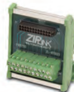
ZL-RTB20 20-pin feed-through connector module
