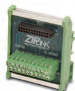
ZL-RTB20 20-pin feed-through connector module
