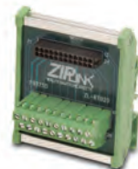
ZL-RTB20 20-pin feed-through connector module
