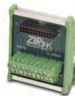
ZL-RTB20 20-pin feed-through connector module
