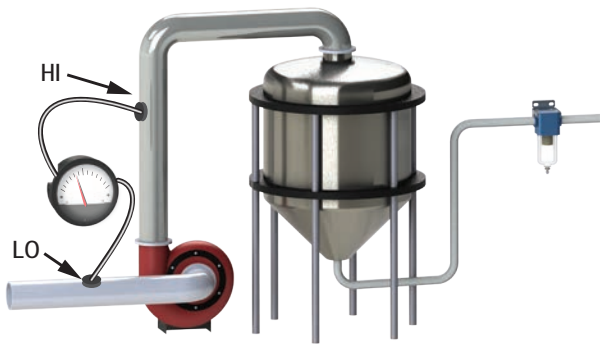
Air/gas flow as a function of blower static pressure
