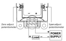
DN-3PLUGMN can be used as a replacement terminal block.
